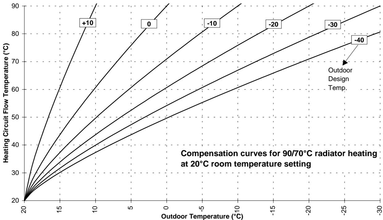
The figures in the boxes on each curve represent the design temperatures which are the expected lowest outside air temperatures of the climactic area where the T3001 controller will be installed.
